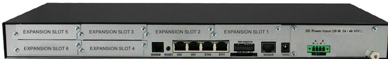
Slot number arrangement (using the SiteBoss 550-6 as an example)
